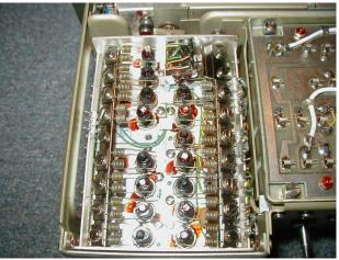
Starting with a connector labeled "Alim 24" mounted to the side of the accessory box, I used my ohmmeter to trace some of the wiring. I eventually decided that, on the basis of these measurements, the radio case was a negative ground, and that three pins on the power connector must receive power. I removed the RF amp and its cabling from the radio
