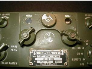
I was curious about a knurled knob on the face of the transceiver. It was embossed with a curly symbol, reminiscent of a lamp filament. I presumed it might have something to do with a pilot or dial light. I unscrewed the knob, and found an empty lamp socket beneath it. I replaced the bulb and turned the radio back on. The circular windows in which the frequency is displayed lit up. So far, so good.
