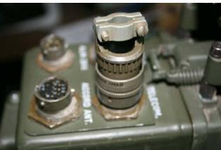
To work around this, I fashioned a jumper composed of an inch of wire with a gold connector pin soldered on each end. The jumper was installed between pins (E) and (G) on the "TELECOM" connector. To protect the jumper, I took a PT06A-12-8P and drilled out its center, leaving only the hollow shell. This *will* fit the TELECOM connector and acts as a tough cover for the jumper.
