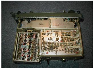
Predictably, the interior exhibits high quality construction. Most of the electronics associated with the radio is housed in small, silver-plated metal modules that plug into to the set. Wiring harnesses are neat, short, tight, bundles. Of course, while this type of construction makes for a rugged set that is easy to service in the field, it makes reverse engineering exceptionally difficult.
