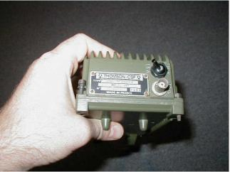
The outboard RF amplifier was attached to the left side of the transceiver. A short length of coax fed the amp from the BNC connector on the face of the transceiver. At the rear of the amp is a short but fat pigtail that links to the accessory module. This must be the conduit through which power and control signals are applied to the amp.
