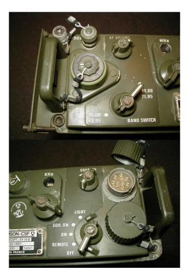
The antenna terminals, which include a BNC as well as a threaded well in which to secure a whip antenna, are located towards the left side of the control panel. At the right of the panel are two circular connectors, identified by Sgt M as "U-79" connectors. (Note: The U-79 is a panel mount connector. The mating connector is called a U-77.) Obviously, these are connection points for the operator's headset.
