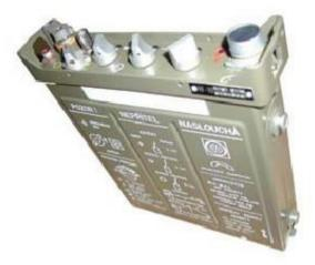
The RF 10 is a radio made by TESLA Czech. This radio has been designed to provide command communications at battalion and company level for dismounted troops. It is used in vehicles by mounted troops
