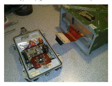
Remove the four screws on the front panel and gently pull away from the case.
