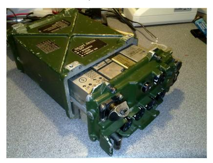
Locate module 13 and with a small flat blade screw driver slowly turn the pot marked R9 anti clockwise until it stops.
